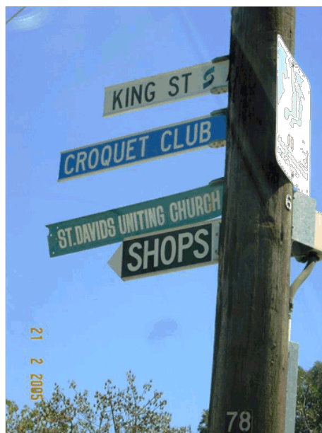
Photo 18 – Croquet Club sign is too close to street name sign. Inconsistent style of community facility signs. Community watch sign partially obscures street name and community facility signs.
