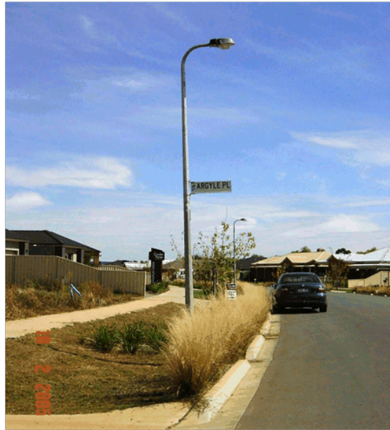
Photo A – Good use of street lighting pole instead of separate pole.
