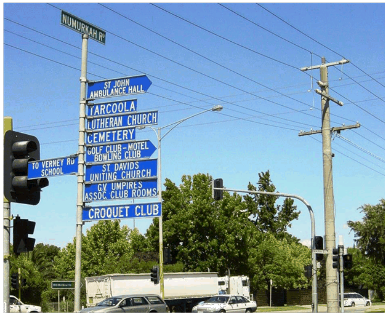
Photo 23 – Too many community facility signs, inconsistent style. Numurkah Road sign is duplicated on power pole in background. A maximum of three community facilities signs is suggested.
