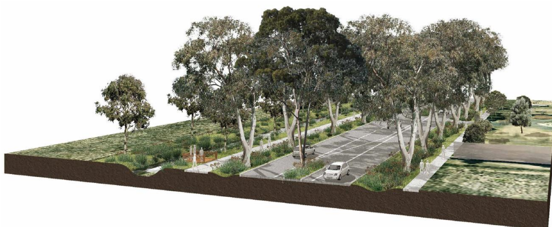
Figure Eight: Proposed Ford Road Cross Section – 27.4 metres (mid-block between Goulburn Valley Highway and Verney Roads).
