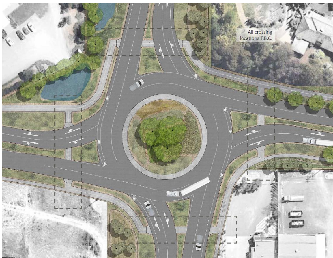
Figure Nine: Concept Plan for the upgrading of the Ford Road, Goulburn Valley Highway and Wanganui Road intersection.
