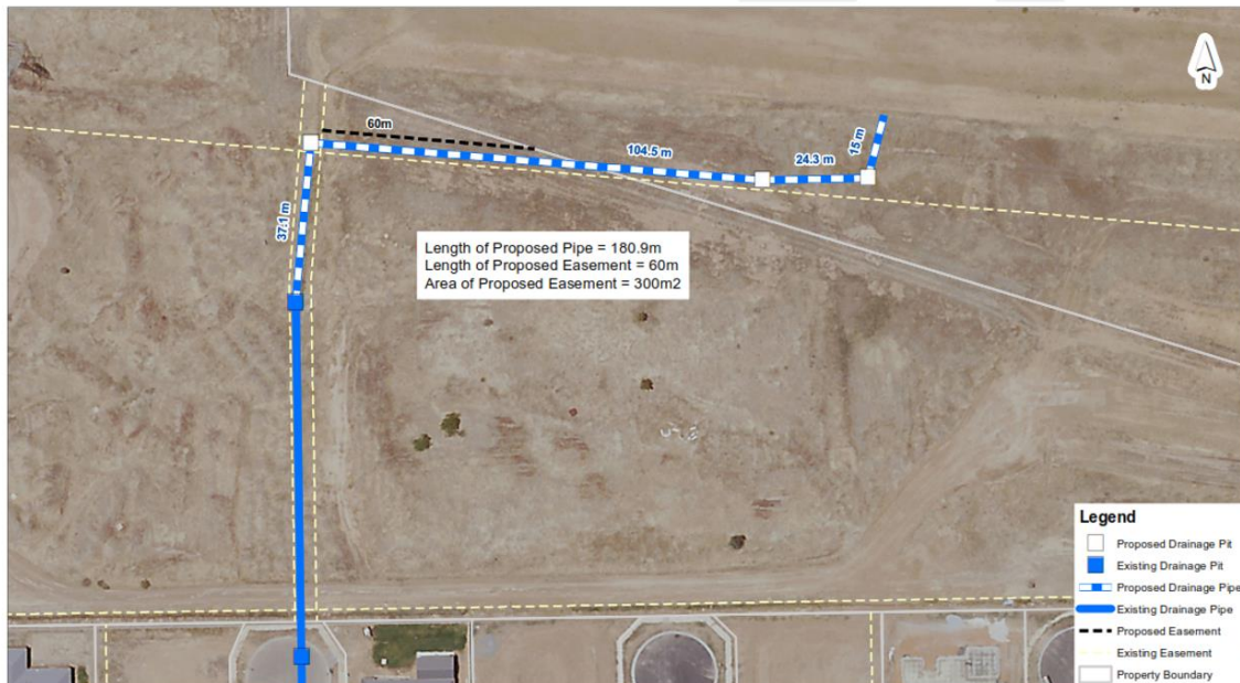
Figure Three: Proposed Drainage Easement.
