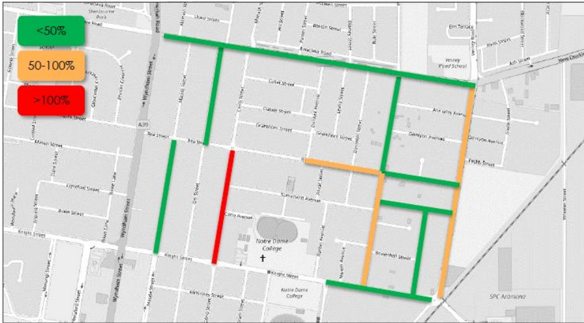
Figure Five: Traffic volumes in the study area relative to road capacity.
