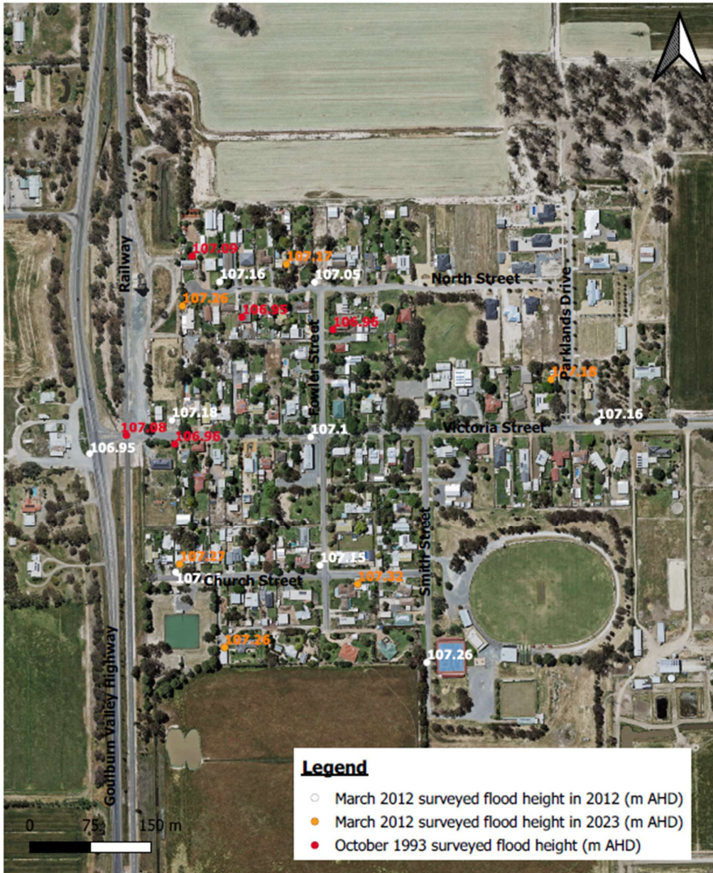
Figure 7 Recorded Flood Height Marks
