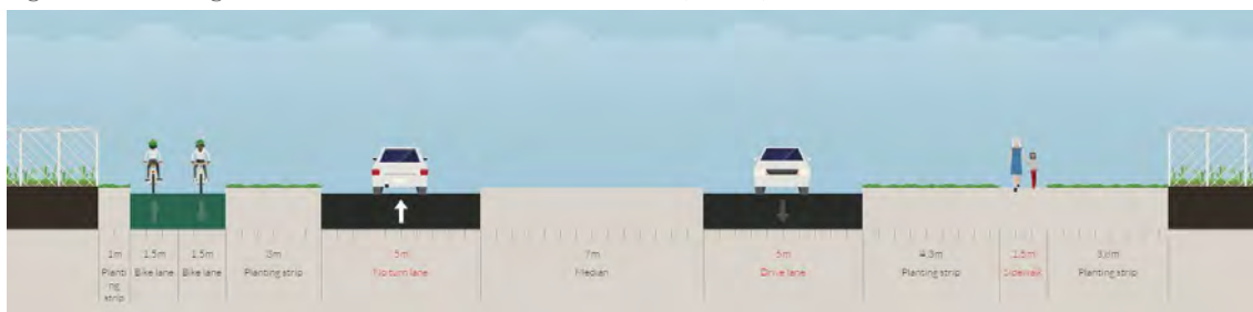
Figure 6.1: Wanganui Road – Mid-Block Cross-Section (33.6m)
