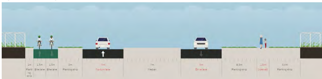
Figure E.1: Wanganui Road – Mid-Block Cross-Section (33.6m)
