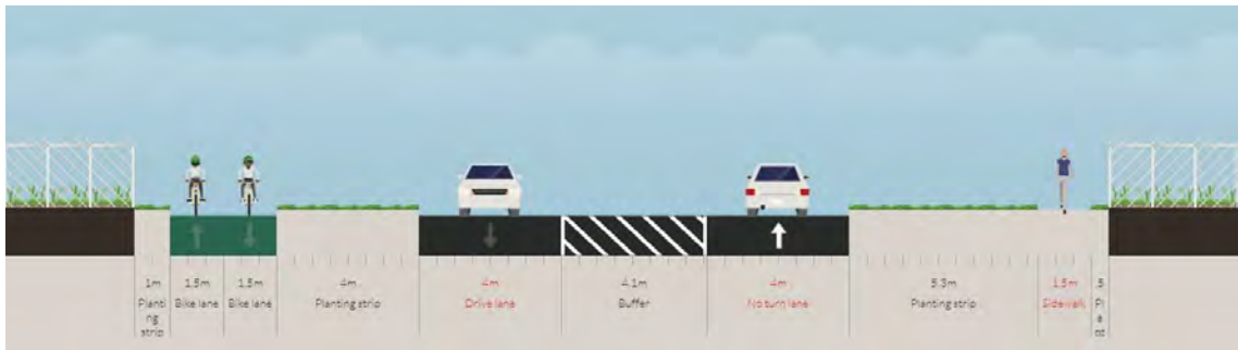
Figure 6.2: Ford Road - Mid-Block Cross-Section (27.4m)
