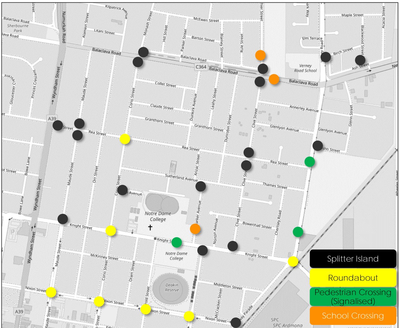
Figure 6 Existing LATM Treatments
