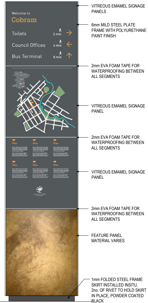
2 TYPICAL PLINTH FRONT VIEW Scale: 1:10
